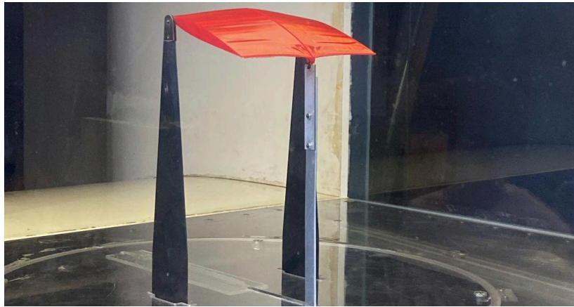
Figure 8: Significant deformation of the most flexible wing model at 35 Hz testing frequency
