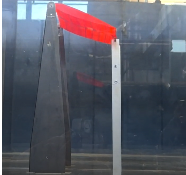
Figure 1: Finite wing mounted to pylons and actuator bar in Boeing wind tunnel
